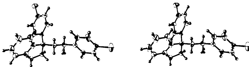
Figure 1. ORTEP stereoscopic drawing of 3c ; 50% ellipsoids were used for C, N, O, and Cl; the hydrogen atoms are shown as 0.15-Å radius spheres.
